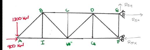
$$F_{ZME=0} ; -1200(16) - 900(3) + R_{FX} (3) = 0 ; R_{FX} = 7300 \text{ KJ}$$
